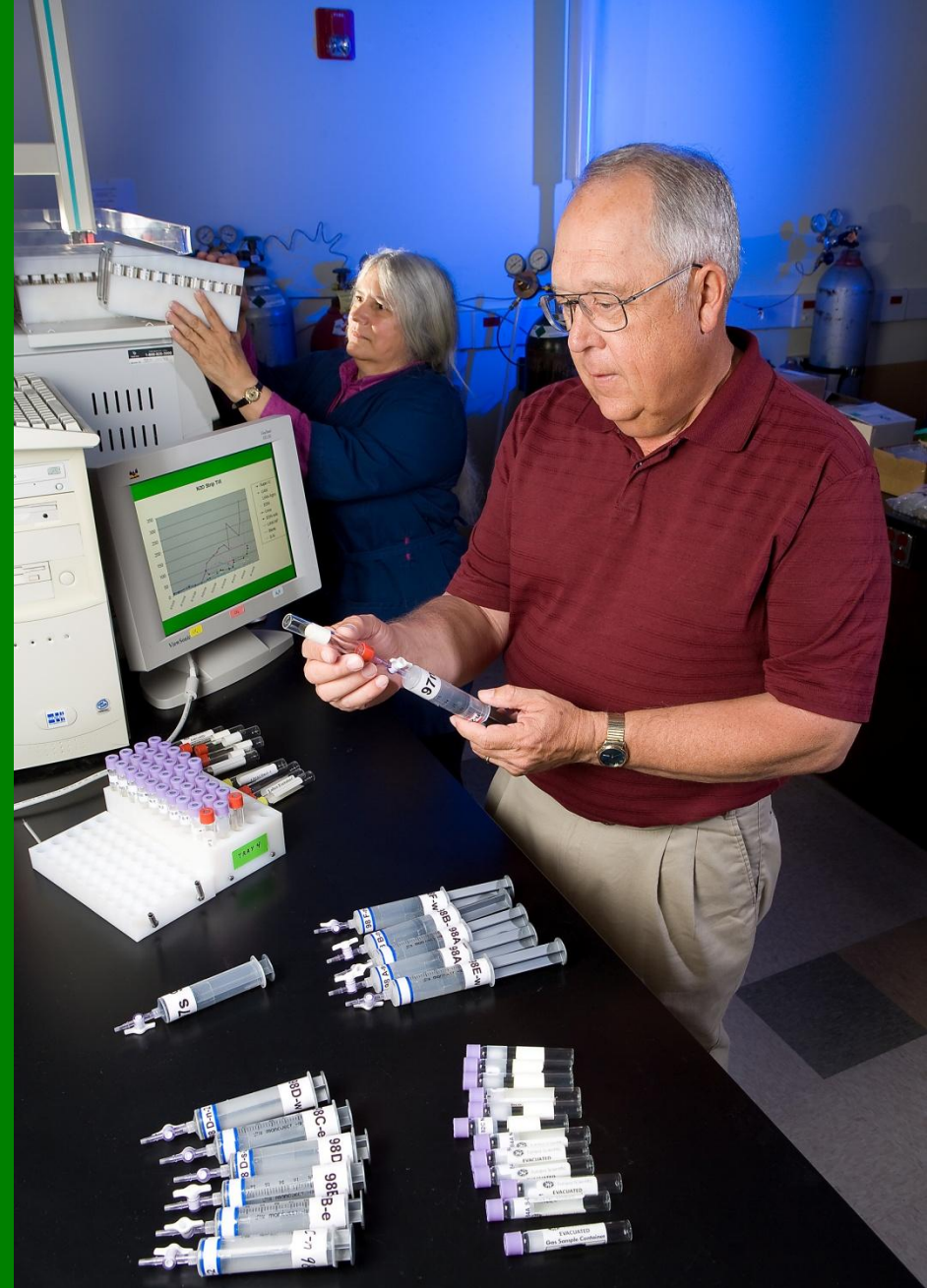
Injecting field gas samples into vials for analysis on Varian 3800 GC.
